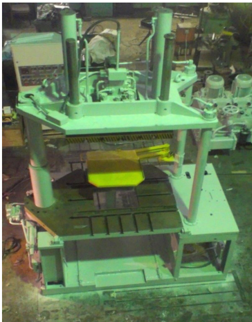
Fig. 3. Low-pressure casting plant U95A model
